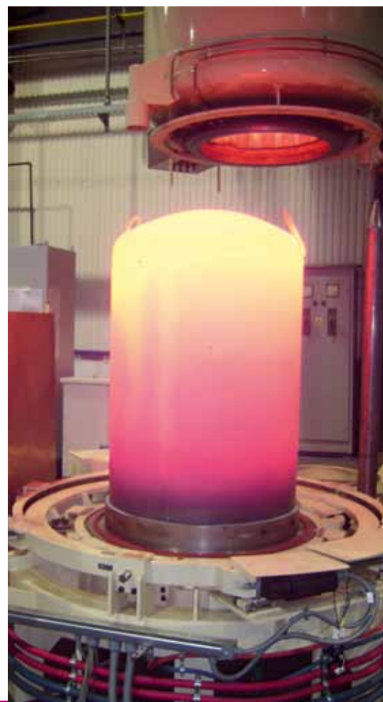
Retort after the CVD process ▶
