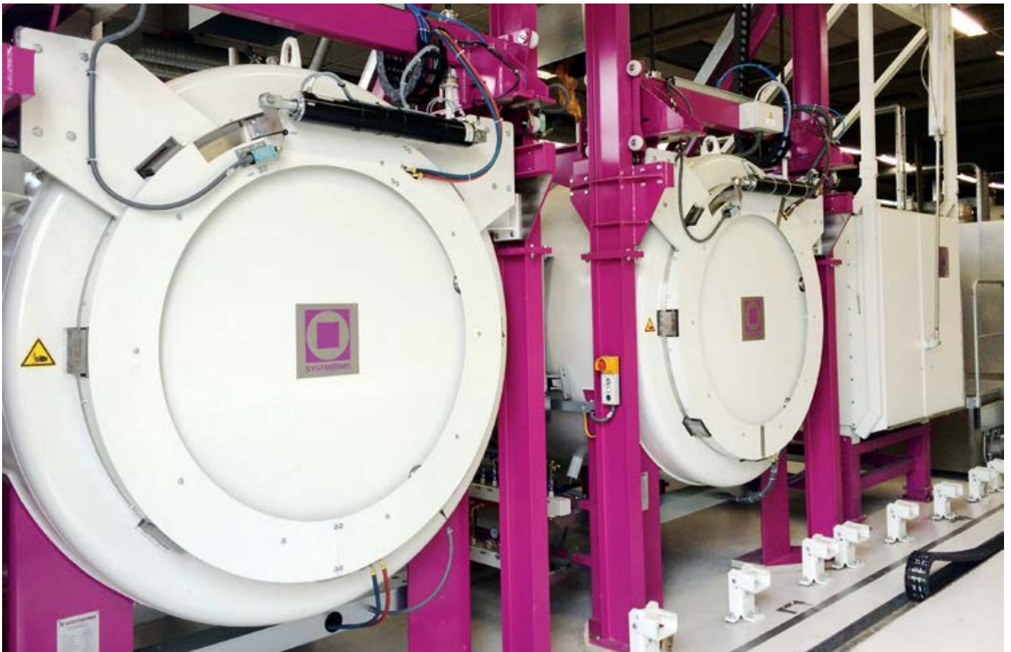
Tempering furnaces with vacuum-tight retort VAN 9812 and chamber furnace LA 9812
